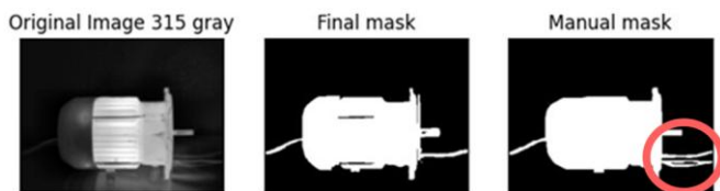
Fig. 7. Comparison between original image, generated mask, and manual ground truth (motor).
