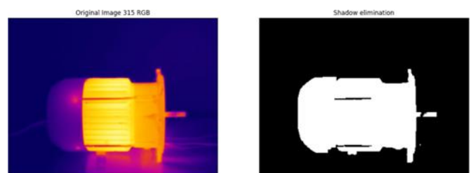
Fig. 6. Enhanced segmentation with shadow removal and morphological operations.
